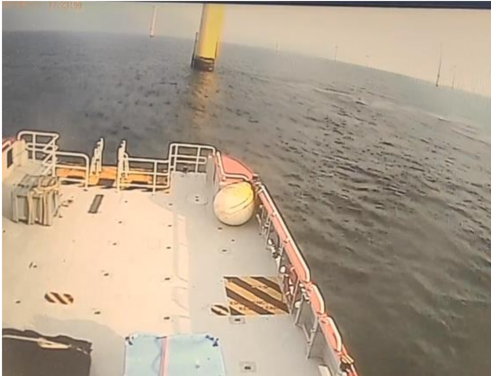
Vessel CCTV coverage showing Njord Forseti approaching turbine tower Q05 shortly before impact. A slick most probably caused by tidal flow can be seen running from the turbine tower across the direction of travel of the vessel.
