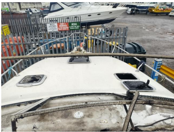
Foredeck port hatch melted starboard hatch opened
