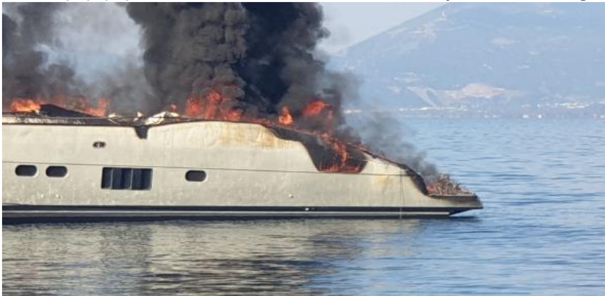
FIG 15 a) b) c) d) accommodation above main deck collapsed, fire full length
