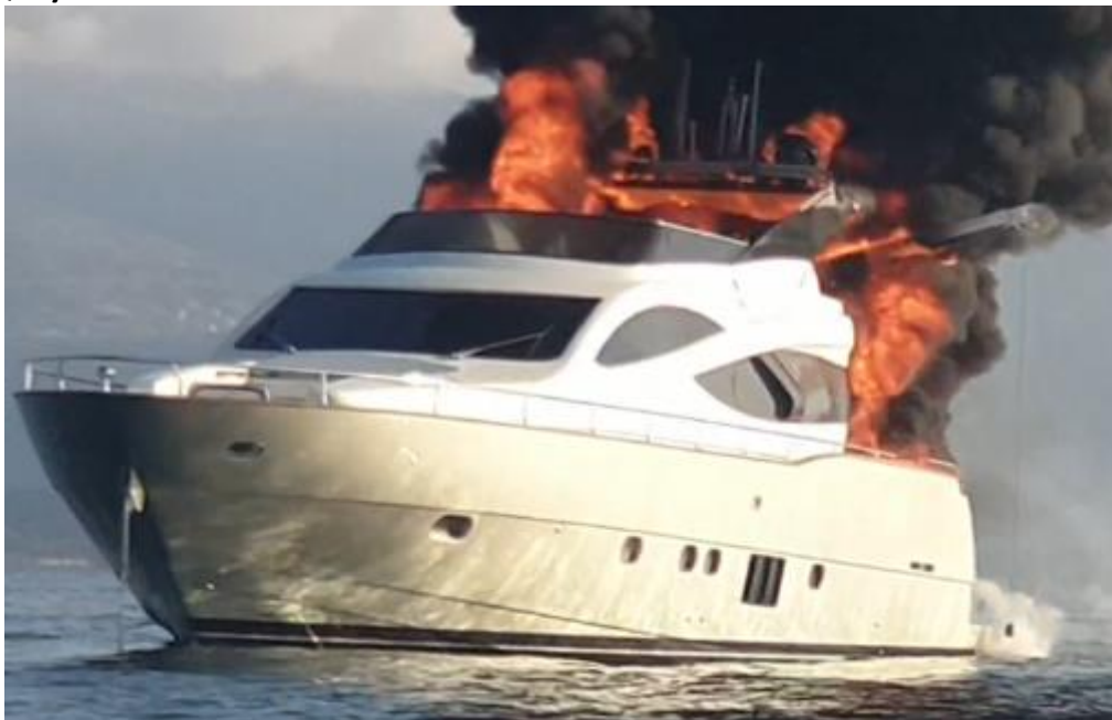
FIG 11 – Fire engulfs the accommodation and spreads to the flying bridge
