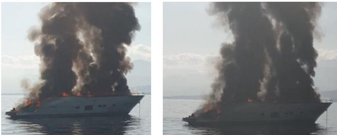
FIG 13 a) & b) Accommodation collapsed and smoke full vessel length
