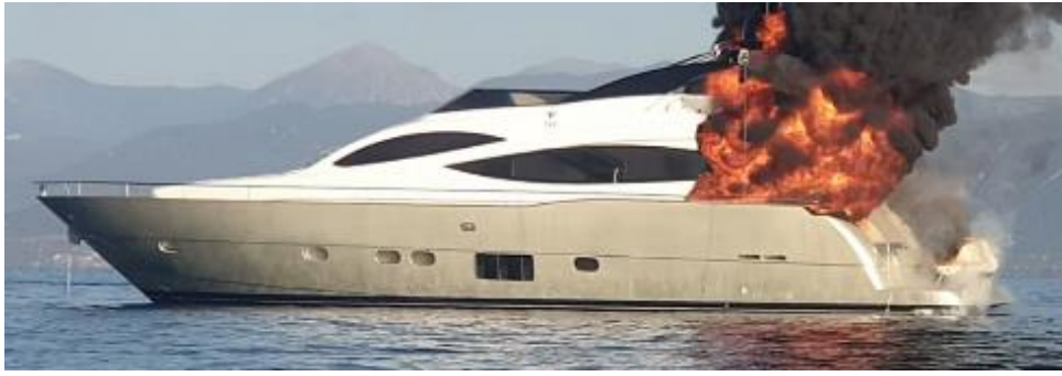
FIG 7- Flames moving forward on Port quarter, cover of PWC catches fire
