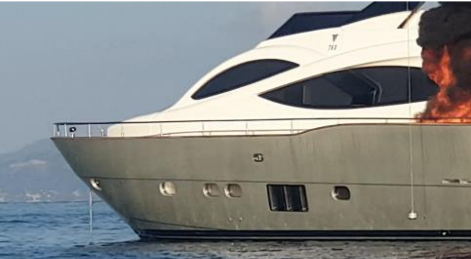
FIG 8 – Port Qtr showing crane wire in position used to deploy tender.
