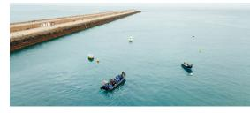
**St Catherine's Harbour** is a deep water harbour, which is situated on Jersey's east coast. The breakwater provides shelter from south-westerly to north winds. The bottom of the harbour is mud/sand, and there is a landing slip at the base of the breakwater.
