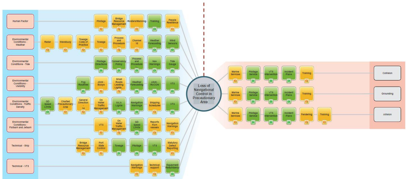
Figure 6 Q Pulse Risk Bowtie, for 'Loss of Navigational control within the Precautionary area'
