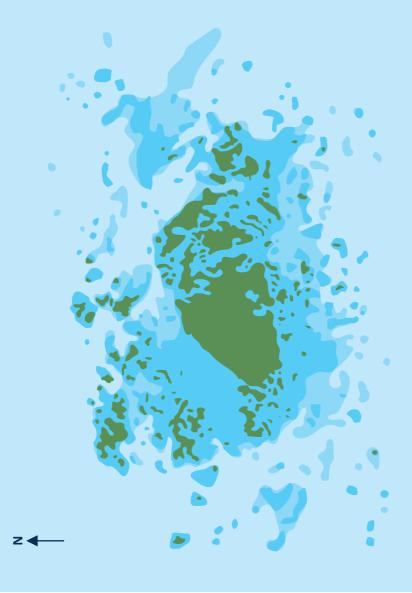
At Les Dirouilles and Les Écréhous, the 10 metre contour line lies outside the pale blue, dark blue and green coloured areas and covers quite an extensive area of these two reefs. The 5 knot speed limit applies in this area to PWCs only. Other craft should keep wash to a minimum.
