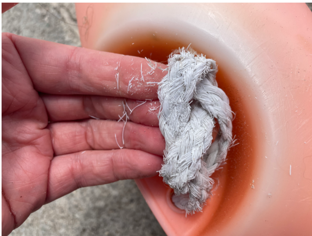
Photo 14. Perishing rope/line on lifebuoy number 018
