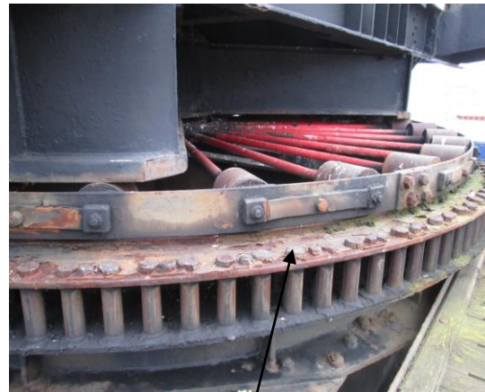
Corrosion on slew bolts and structure surface
