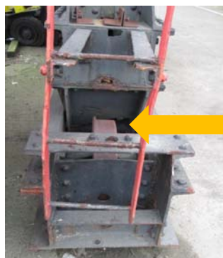
There are significant signs of collision damage to several major elements, other components are warped and twisted, causing considerable Health & Safety issues .
