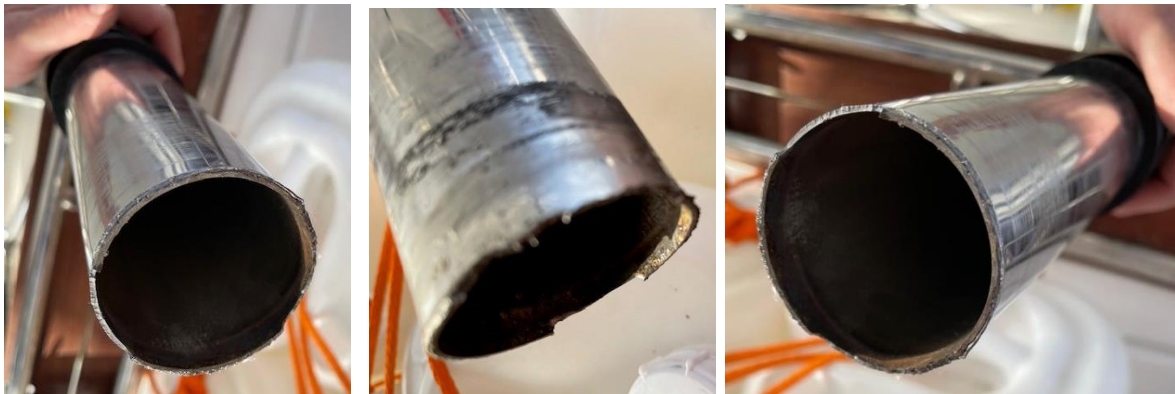
(Fig 4, 5, & 6: bottom of seat support pillar following failure)
