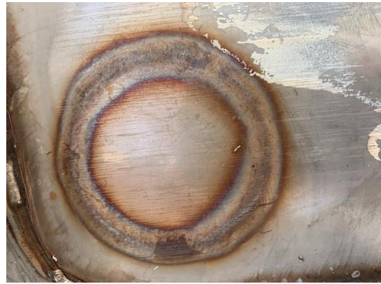
(Fig 3: Crack on underside of base plate)
