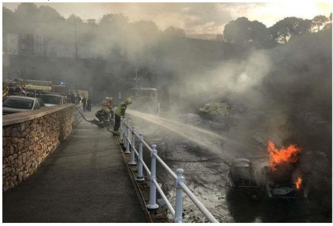
The fire and explosion aboard INNER MEETING were caused when a build-up of flammable vapour from fumes from the vessel's inboard petrol tank and from the spray paint being used in the cabin was ignited by an electrical spark; at a time when work was being carried out in the cockpit on an electric pump.
