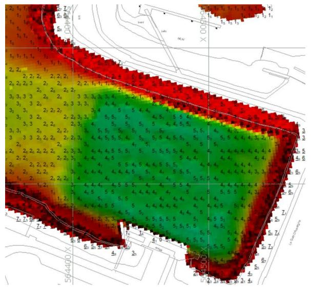
Figure 9 Bathymetry data, Tanker berth with Soundings overlay
