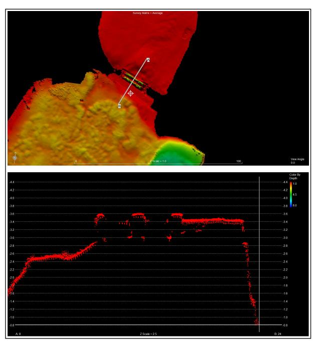
Figure 2 Profile across St Helier Marina Sill, multiply lines of data, showing a height of 3.6m above CD
