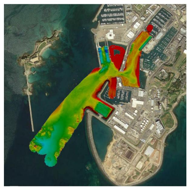
Figure 3 October 2019Harbour survey, bathymetric data set
