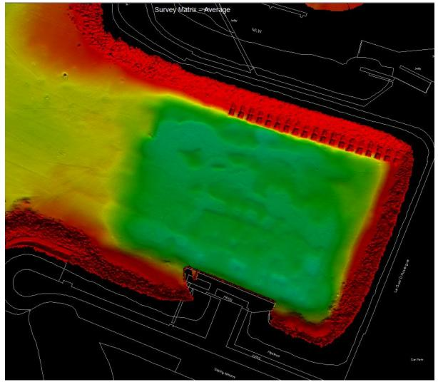
Figure 8 Bathymetry data, Tanker Berth
