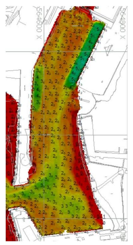
Figure 5 Bathymetry data, St Helier Main Harbour with Soundings overlay
