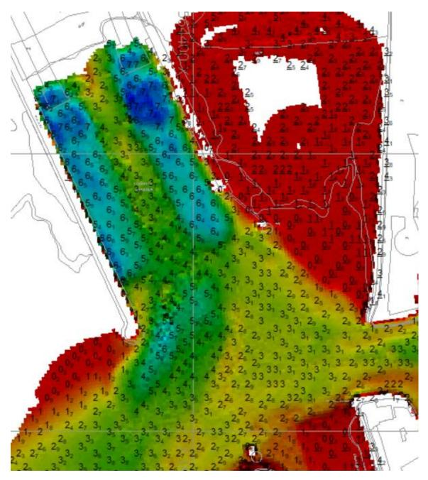
Figure 7 Bathymetry data, East and West Berth with Soundings overlay
