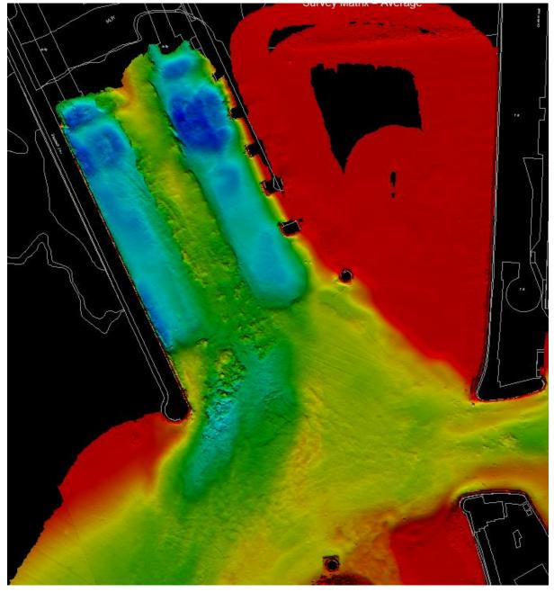
Figure 6 Bathymetry data, East and West Berths
